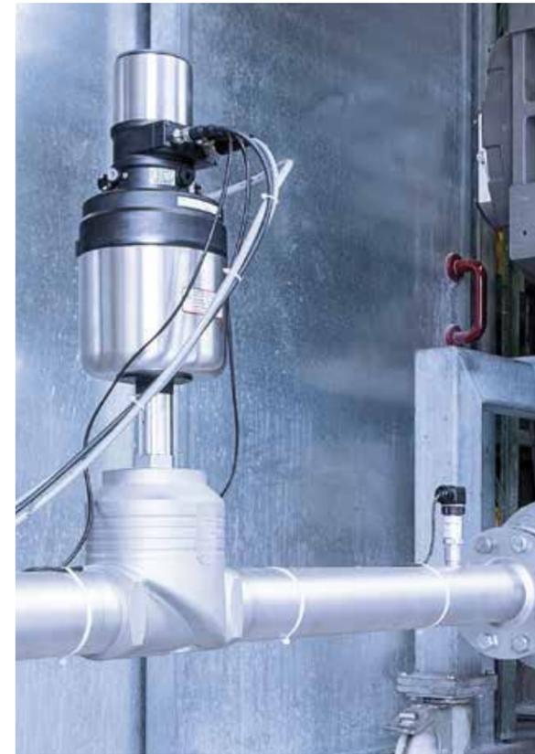
Application of air flow rate controller type 8750 in the conveying system of Zeppelin Systems GmbH
